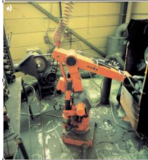
ASEA IRB-6 (1973) first robot all-electric-drives
