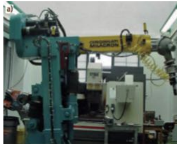
Cincinnati Milacron T3 (1974) first micro- computer controlled robot
