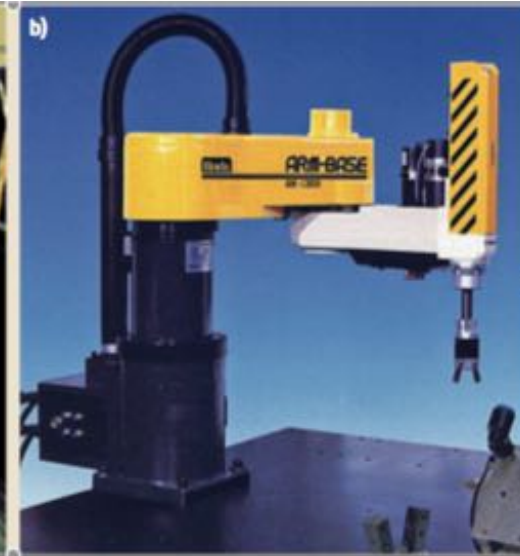
Hirata AR-300 (1978) first SCARA robot
