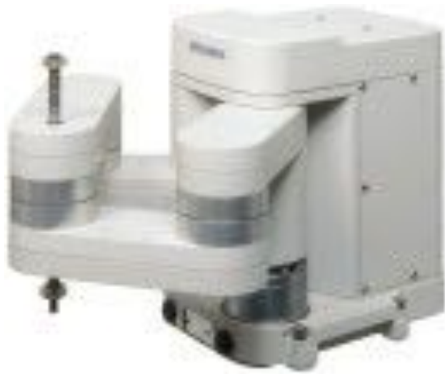
Mitsubishi RP (repeatability 5 micron, payload 5 kg)
