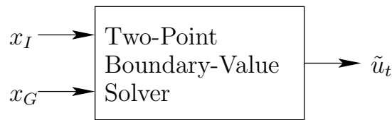
Figure 14.10: Some methods in Chapter 15 can solve two-point boundary value problems in the absence of X_{obs} . This is difficult to obtain for most systems, but it is more powerful than the system simulator. It is very valuable, for example, in making a sampling-based roadmap that satisfies differential constraints.
