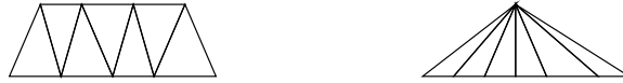
Figure 3.6: Triangle strips and triangle fans can reduce the number of redundant points.
